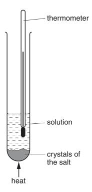
10 g of water was transferred into a boiling-tube. To this 0.5 g of potassium chlorate(V) was added.
